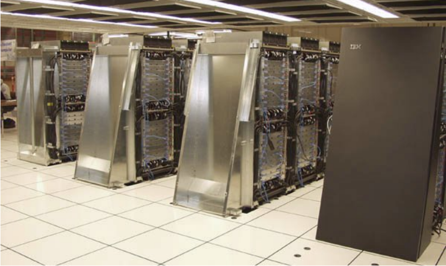
IBM's Blue Gene (pun intended) supercomputer runs a lightweight Linux on each compute node, and a complete Linux on its management nodes.
